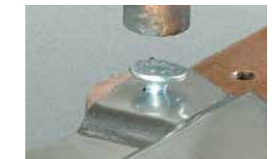
Perfect stud and sheet centring with a sleeve made of VOLCERA
